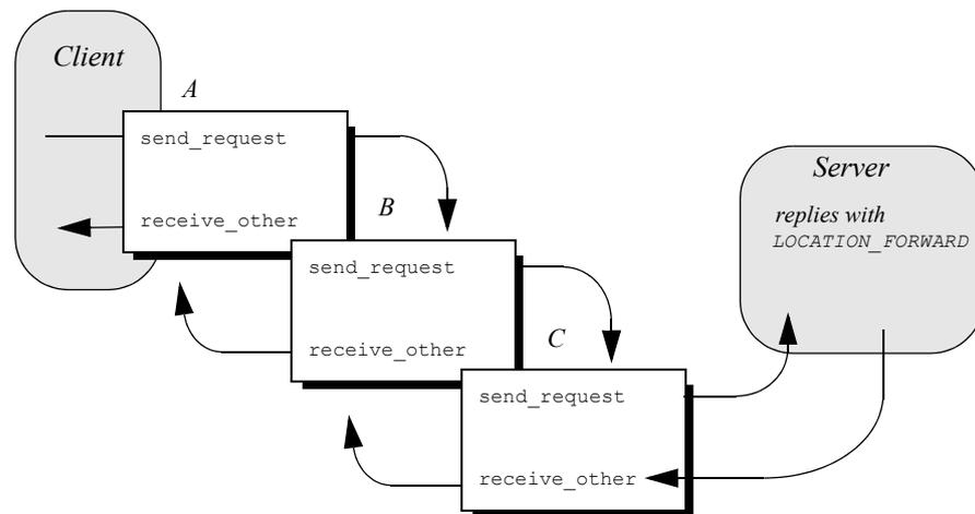
Figure 48 Client interceptors process a `LOCATION_FORWARD` reply.
