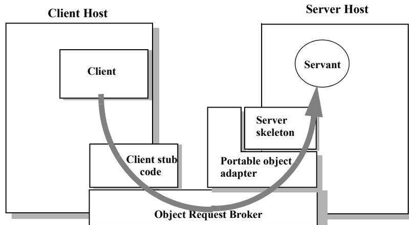
Figure 5 The portable object adapter
