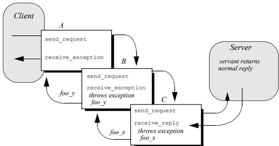
Figure 50 Client interceptors can change the nature of the reply.
