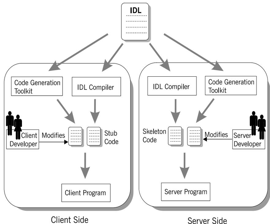
First, you define a set of interfaces written in the OMG interface definition language (IDL). The IDL forms the basis of development for both the client and the server. The toolkit takes the IDL file as input and, based on the declarations in the IDL file, generates a complete, working Orbix application. You can then modify the generated code to add business logic to the application.
