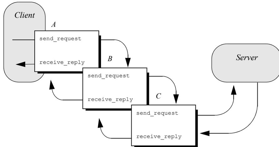
Figure 47 Client interceptors process a normal reply.
