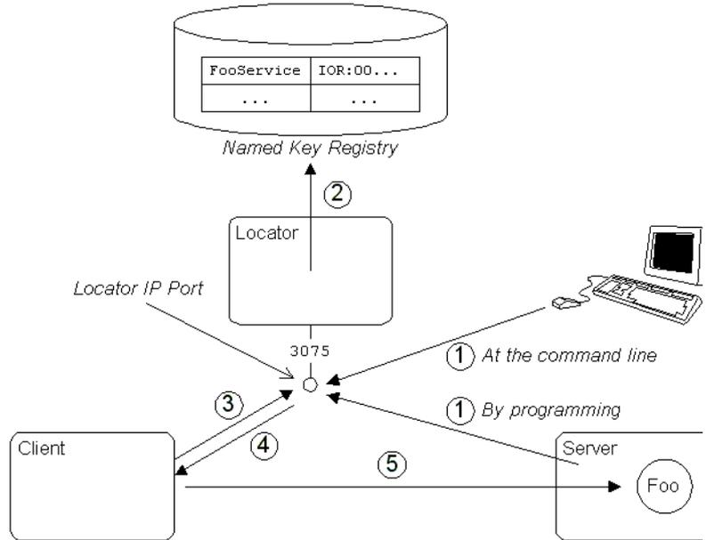
Figure 57 Using `corbaloc` with the Locator-Based Named Key Registry
