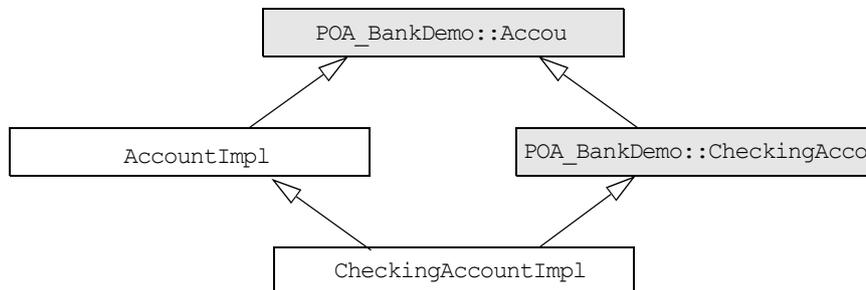
**Figure 18** A servant class can inherit base class implementations.
