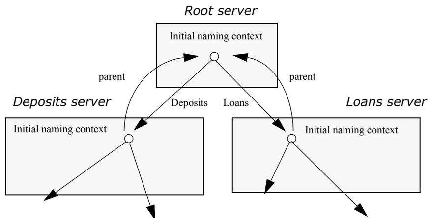
**Figure 31** The root server's initial naming context is bound to the initial naming contexts of other servers, allowing clients to locate the root naming context.
