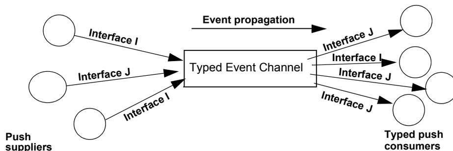
**Figure 44** Push consumers pushing typed events to typed push consumers
