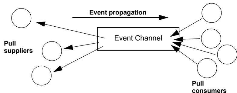
Figure 42 Pull Model suppliers and consumers communicating through an event channel
