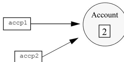
**Figure 18** Reference for Account proxy is incremented to 2.
