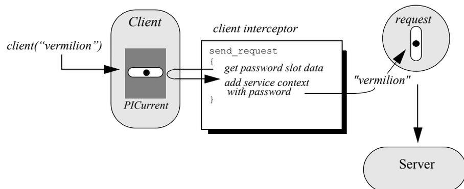
**Figure 46** PICurrent facilitates transfer of thread context data to a request or reply.
