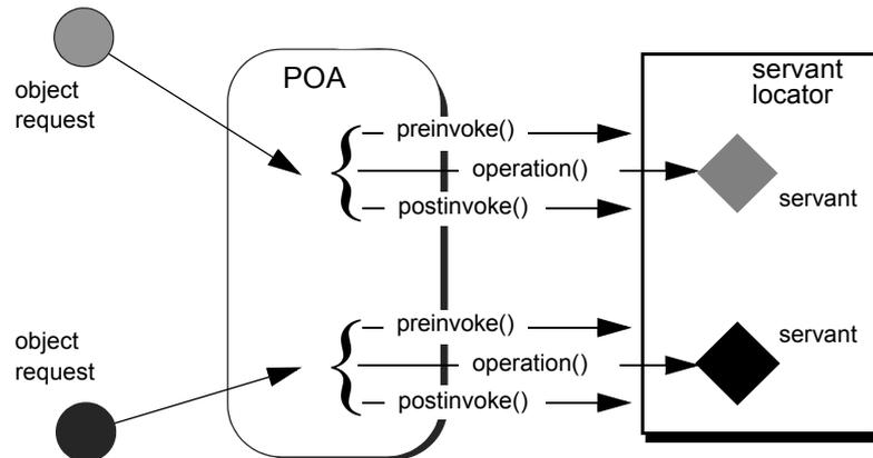
**Figure 20** The POA directs each object request to the servant locator, which returns a servant to the POA to process the request.
