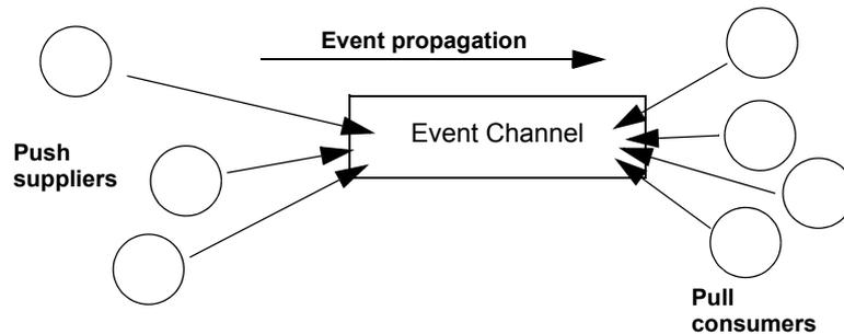
**Figure 43** Push suppliers and pull consumers communicating through an event channel
