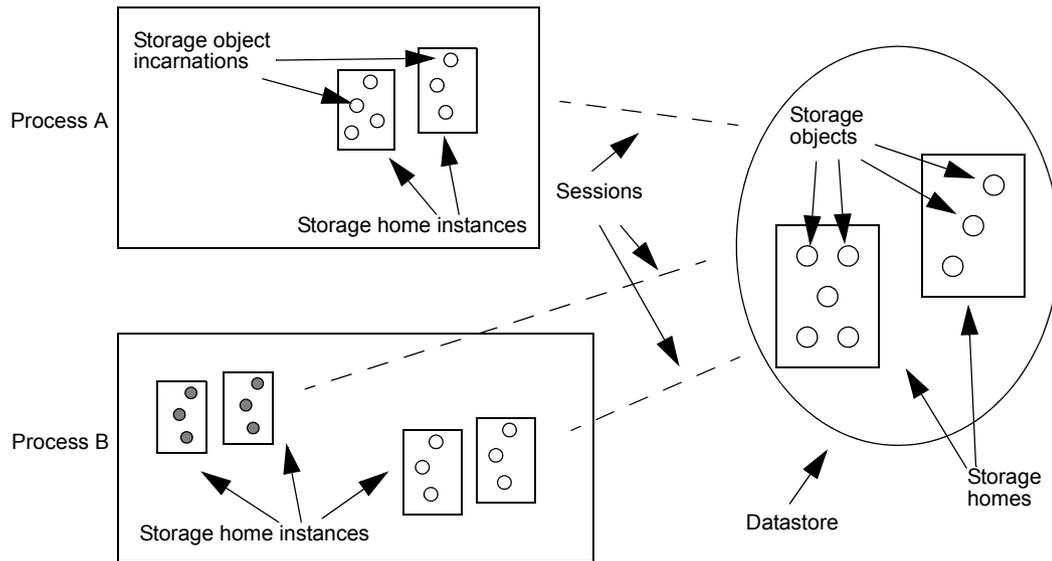
**Figure 34** A server process uses sessions to establish a logical connection with a datastore and its contents
